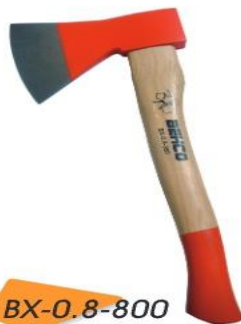
BX-0.8-800 800 g Feuerwehrraxt Axe • Head material : 1055 medium carbon steel • Head finish : orange baked paint finish, edge polished • Handle : natural color hickory handle with pad print
